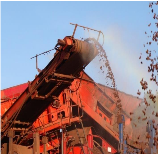
Photo-2 Mobile screen Plant Equipped with dry fog system for dust suppression
