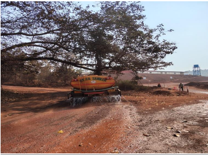
Photo-6 Water sprinkling through mobile tanker on mineral transport road adjacent to mines lease.
