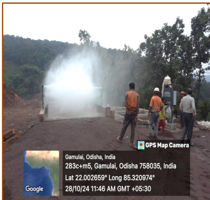
Photo-3 Wheel wash facility at the exit gate of Mines with recirculation system
