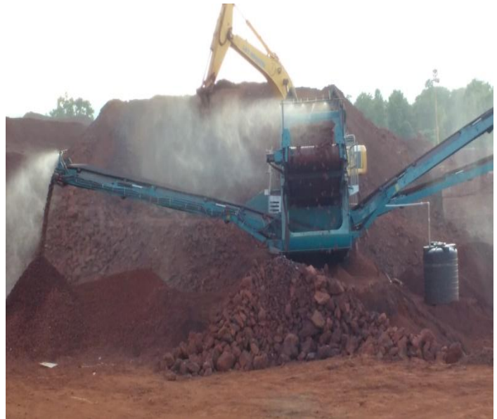
Photo-2 Mobile screen Plant Equipped with dry fog system for dust suppression
